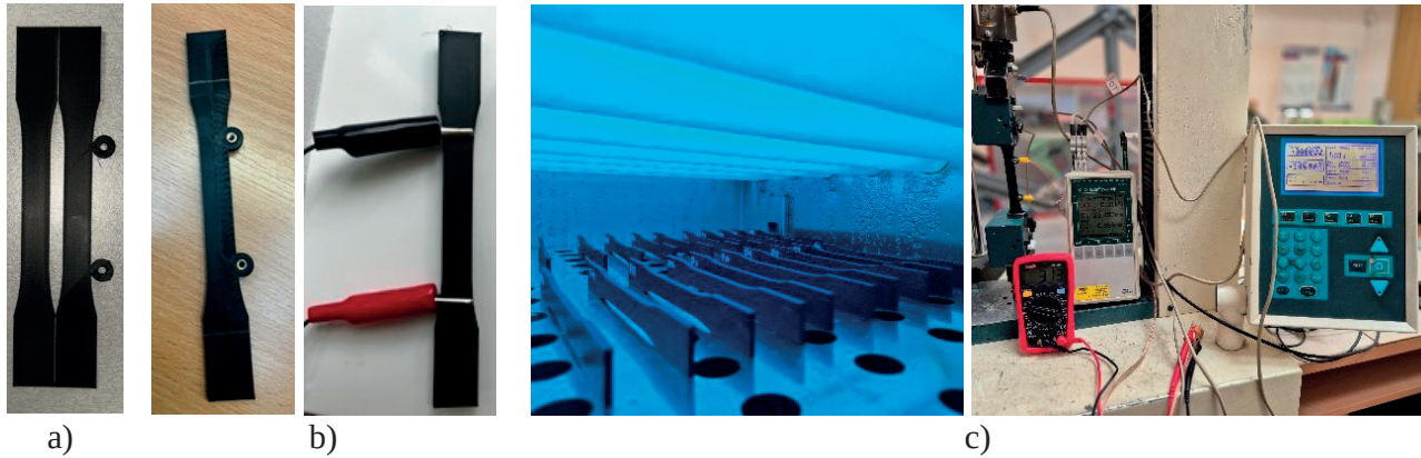
Figure 1. Experimental programme: a) 3D-printed tensile specimens, b) modified conductive PLA specimen with brass inserts and clip contacts, c) experimental setup of specimen conditioning and tensile tests.
